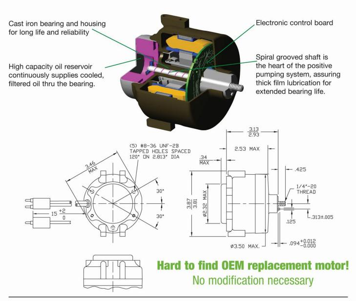
"The iMotor refrigeration motor uses less wattage to achieve the same airflow as a shaded pole motor, so it produces less heat. Fewer BTU's in the system means less work and wear for the compressor for even greater savings."
