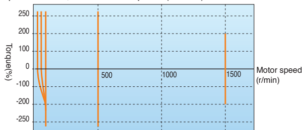
Example torque characteristics [5.5kW]
