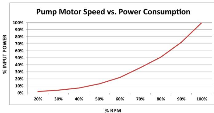
This graph shows the large increase in energy consumption when running the pump and motor at high speeds. Slowing the pump and motor speed saves significant energy dollars, similar to better automobile gas mileage when driving 40 mph versus 70 mph.
