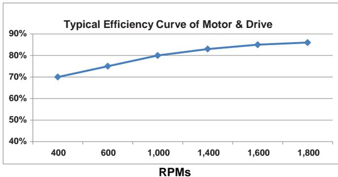
Traditional commercial duty pumps run at only one speed and the one speed is high speed. Most pumps are usually oversized for the application and they rely on induction motor technologies which are far less efficient than ECM technology. This results in traditional pumps being energy hogs. ECM technology can save commercial building owners 30% to 90% in energy savings.
